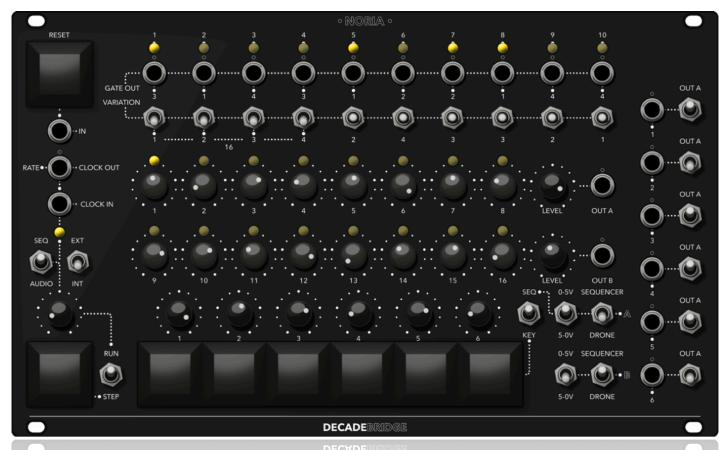
**NORIA** is an old skool style 16 step analog sequencer and can also be used as a drone/glitch/pseudo self sequenced synth. It can be installed into your eurorack case or used as a standalone controller/instrument.
