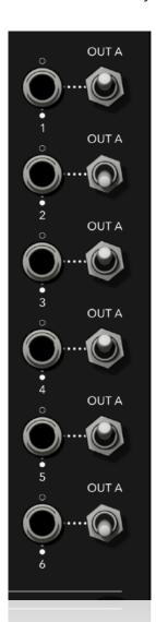
The 6 outputs and relevant switches to the right of NORIA set the keys (above) output destination. If the switch is in the up position the the key is routed to 'OUT A' (dependent upon the 'SEQ/KEY' switch above).
