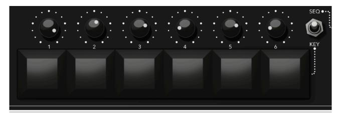
The switch to the right sets the source for 'OUT A' (see previous page). In the up position 'OUT A' will take the signal from the sequencer. In the down position it will take the signal from these 6 keys. The output voltage for each key is then set using the relevant knob above the key (1-6).
