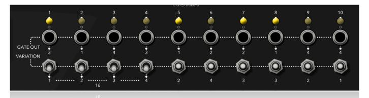
**NORIA**'s variation switches can be found underneath the 10 gate outputs. These can be used to quickly change up the sequence and rate of the instrument. These can also create interesting variations when running **NORIA** at audio rate and using it as a drone synth.
