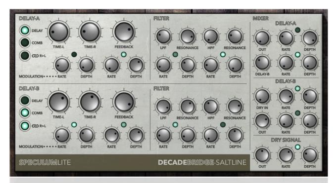
SpeculumLite is a dual delay line/comb filter effect that can create a wide range of sounds ranging from ambient echoes and reverbs to modulated, glitchy delays.
