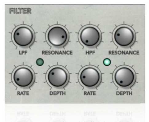
The signal from the delay section is passed through the filter. The signal is fed through a resonant low pass filter first and then through a resonant high pass filter.
