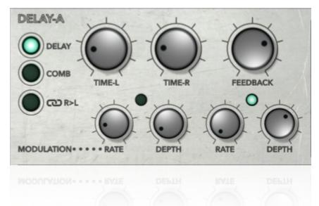
SpeculumLite's delay lines are a simple affair. The buttons to the left of this section determine the 'TIME' range of the delay. 'DELAY' repeats the incoming signal like a standard delay effect. 'COMB' runs at a far quicker rate to create a comb filter effect. The 'R>L' button links both the left and right delay rates. With this on, 'TIME-L' changes the delay time of both channels.
